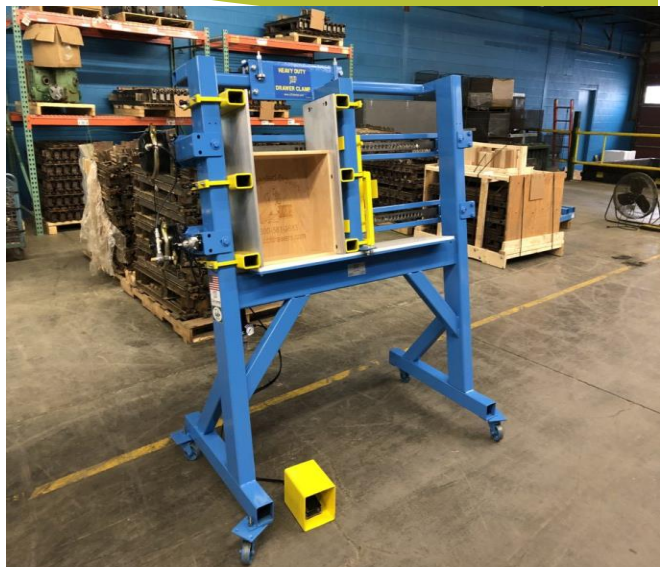
JLT #190B-M3-48 Drawer Clamp 12" x 24" x 48" Capacity Fast Acting Cylinders
